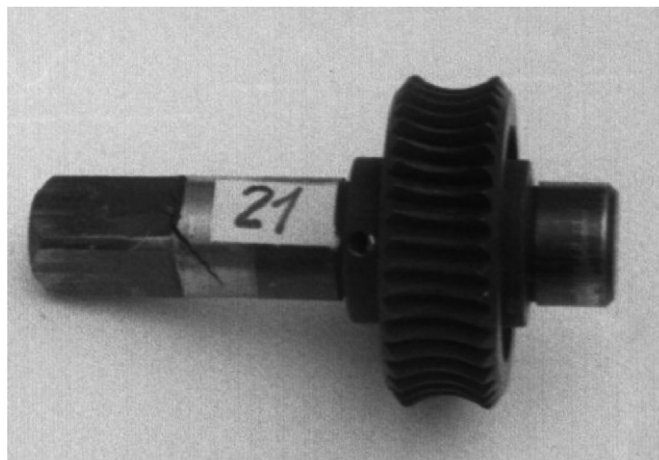
Fig. 10. Cracked shaft under torsional impact fatigue.
